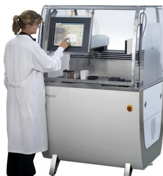
The state-of-the-art automated QPatch-HT system (48 channels) enables higher throughput, lower cost, and better consistency for hERG channel recordings
