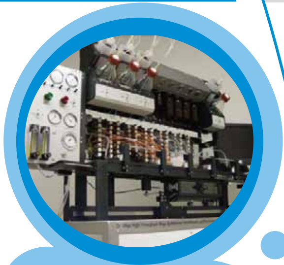
Dr. Oligo 192 DNA Synthesizer For high throughput oligonucleotide synthesis
